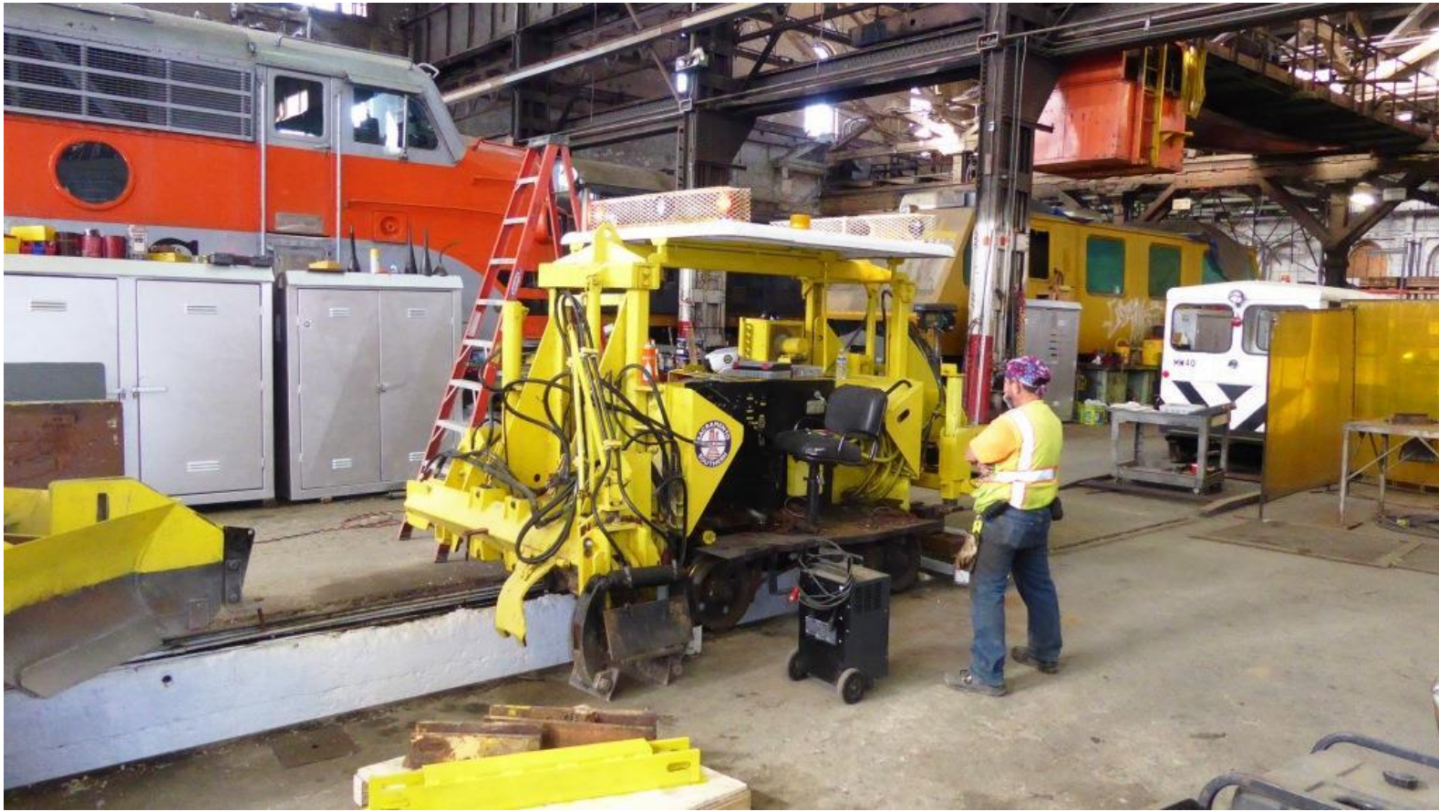
Joe fires-up fully rewired Jackson 125 tie-exchanger and looks at it approvingly
