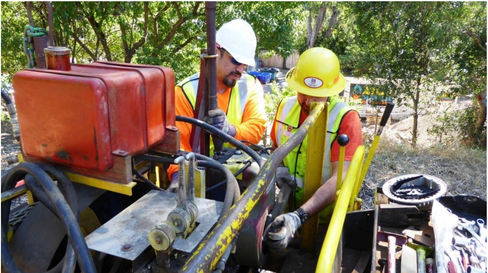
Jose and Chris M. improvise a solution to the malfunctioning pull-start by wrapping a strap around the start-wheel
