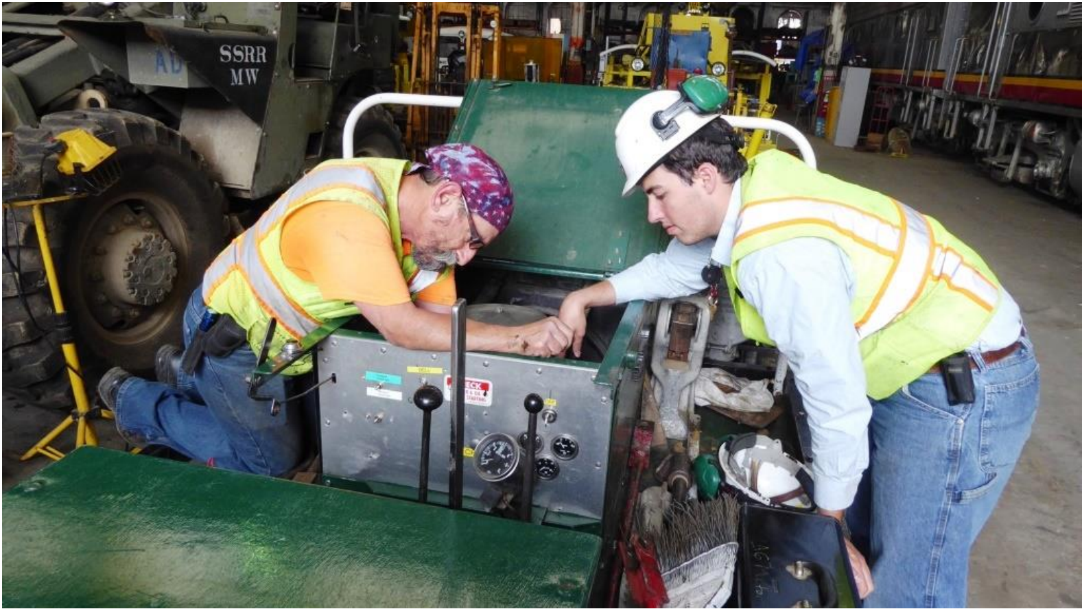
Joe and Weston rewire the radio into the ignition switch of the A-6 motorcar
