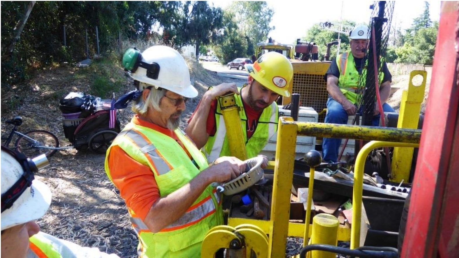
Ed and Chris M. remove the cowling on the mechanical gauger's pull-start after it pulled-apart...
